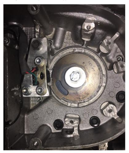
The trigger wheel from Ignitech has pilot hole, which needs mounting to a taper mount for the crank.
